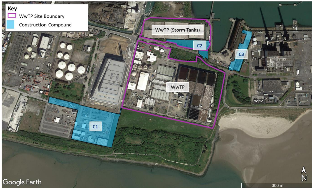
Figure 3-8: Construction Compound Areas
