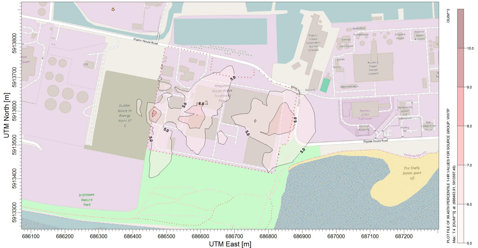
Figure 10-7: Predicted Odour Concentration - Ringsend Project Odour Goal - 'Post-Development' Scenario - ou_E.m^{-3} as the 99.4 th percentile of hourly averages 2014
