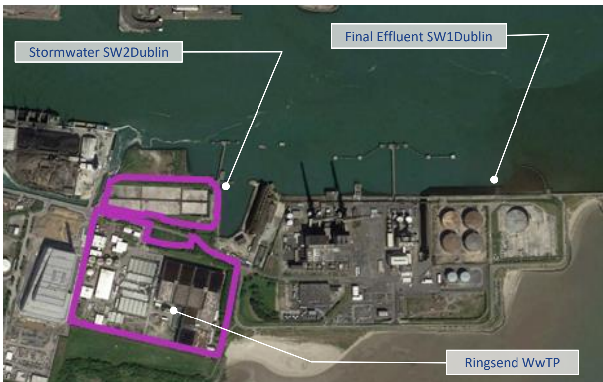
Figure 4-9: Wastewater Discharge Locations
