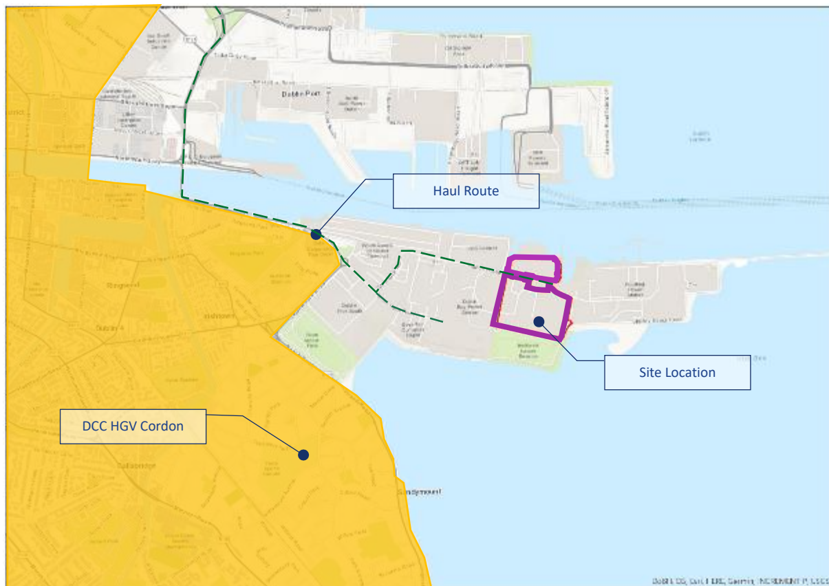
Figure 13-3: Dublin City Council HGV Cordon Area in relation to site and proposed HGV route
