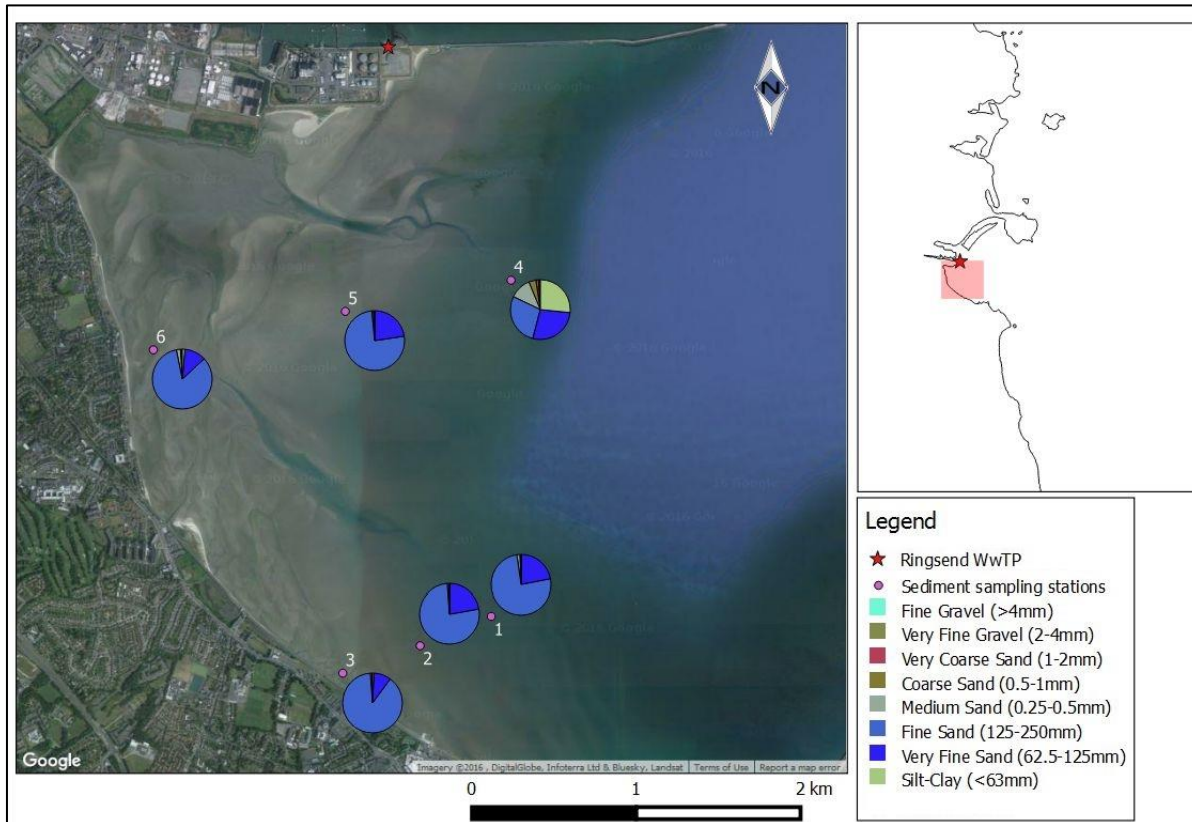
Figure 5-8: Results of granulometric (PSA) analysis for sediment samples collected from stations in South Dublin Bay
